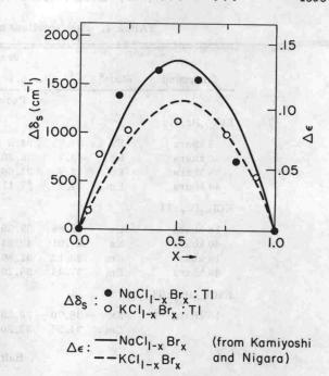
FIG. 2. Deviation of Stokes shift and dielectric constant from linearity with composition—NaCl<sub>1-x</sub>Br<sub>x</sub>: Tl and KCl<sub>1-x</sub>Br<sub>x</sub>: Tl.
